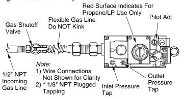
Figure 21 - Connecting Flexible Gas Line to Millivolt Valve
